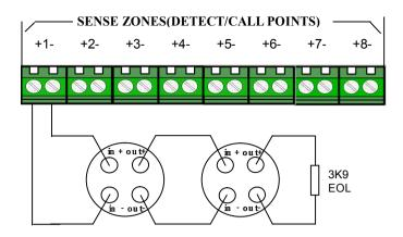
Figure 2.3 - Detectors Wiring Connection
