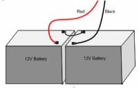
Figure 2.2 - Batteries Wiring Connection
